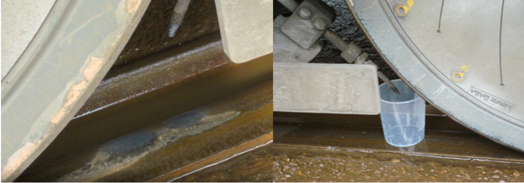
Measuring the quantities sprayed onto the railhead.
